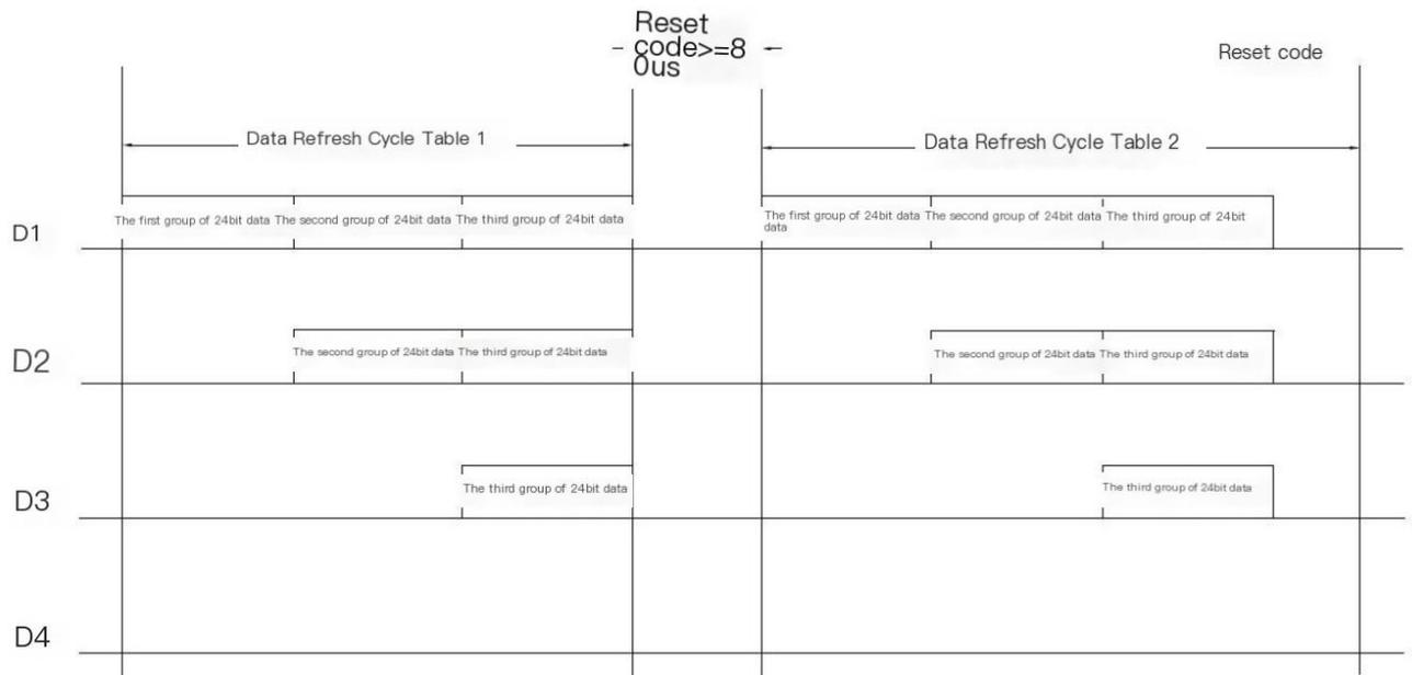
Note: D1 is the data sent by MCU, D2, D3 and D4 are the data automatically shaped and forwarded by cascade circuit.
