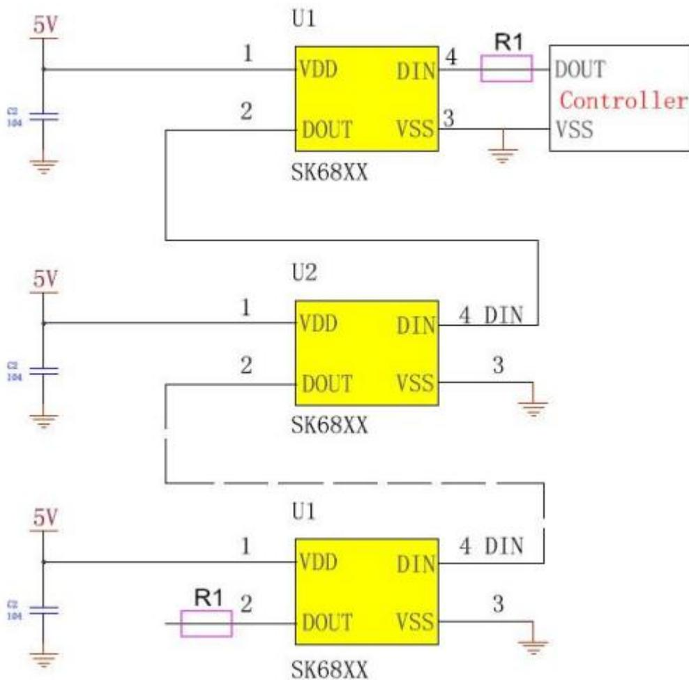
In the actual application circuit, in order to prevent the instantaneous high-voltage damage to the IC internal signal input and output pins caused by hot plugging during the test
