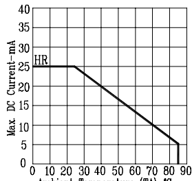
Fig5. MAX. ALLOWABLE DC CURRENT VS. AMBIENT TEMPERATURE.
